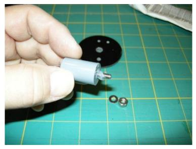
(7) When mounting the Eye use a liberal amount of Blue Threadlocker (Medium Strength) on the exterior nut. I use high strength (Red) theadlocker on any items that I do not intent to ever separate. This will prevent the nuts from unscrewing. Again use Silicone Caulk around the threads and washer when mounting to the bulkhead to prevent blow back from the charges.
