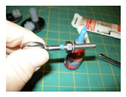
(8) Here is a completed bulkhead. You can see some caulk around the Charge Well. I let these sit till the caulk and threadlocker have setup.
