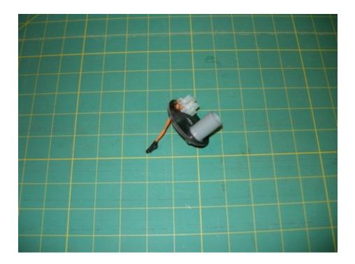
(3) The other bulkhead is the removable one and is wired up the same way. The wire is trimmed to just what is needed.
