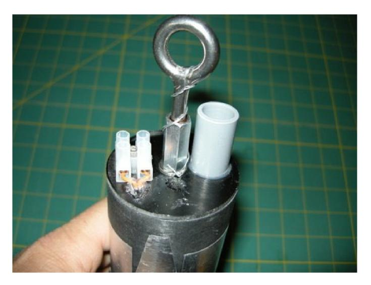
(9) For the removable end, you can see the lug to run safety wire through. Notice that the safety wire is wrapped around the Eye and steel coupler and secured to the lug in the direction that prevents the Eye from unscrewing. It just takes seconds to do, so I replace this wire after each flight.
