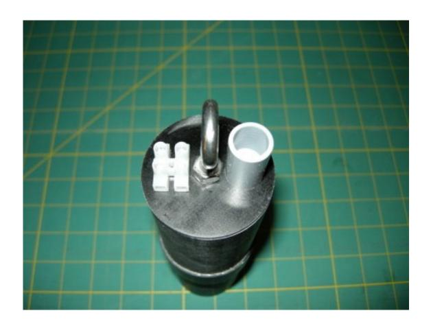
(1) Lay out the parts on the bulkhead. We are using Dog House Rocketry 2position Terminal Blocks and 1.5g Charge Wells. My preference is to have the Charge Well and Terminal Block on opposite sides to give me room to work with. As you layout the parts keep in mind that there is mounting hardware on the interior and you want to ensure that does not interfere with the coupler.
