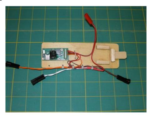
(7) Here is the completed assembly. A couple of 1/420 nuts are used to hold the tray in place one acting as a lock nut. The white connector will hook to the switch connector mounted in the coupler. The basswood tab prevents rotation. The battery will be secured using electrical tape.
