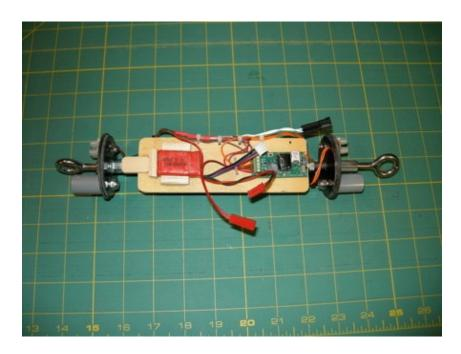
(8) Here is the installed assembly. The right side is the removeable bulkhead and the assembly is installed from the left. Note I have add mounting holes for securing the forward body tube and have added metal tape to tighten the fit with the sustainer tubing.
