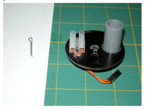
(4) I have modified the removable bulkhead to have a small tiedown using a cotter pin. Since this bulkhead will be removable, I will use safety wire to prevent the large Screw Eye from inadvertantly unscrewing in flight or while spinning under a chute.
