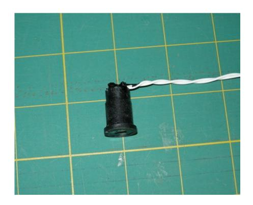
(1) I am using the Rotary Switch that came with the kit so I drill a 1/2" hole into the Switch Band. I prefer to use a Forstner Bit because with a little practice it tends to cut a cleaner hole. I like to keep the Bay uncluttered so I trim the switch wire so when the switch is installed the connector will stick out an inch or two from the coupler. I use white wire for switches.
