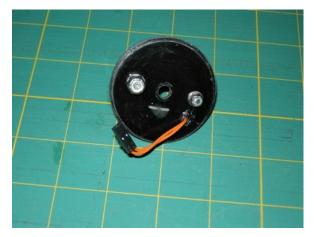
(6) I made the altimeter tray from a piece of 1/8" ply. I am using an Aluminum tube and balsa triangle stock with epoxy to secure the tube on the back side. I have drilled holes for the Altimeter and wire ties.
