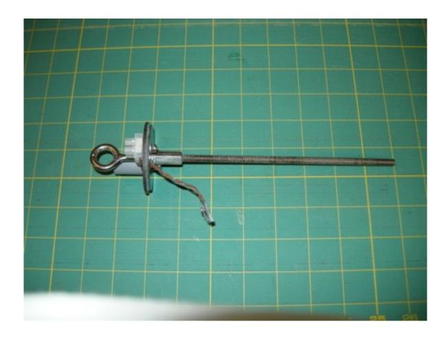
(2) I assembled one end by securing a steel threaded coupler and threaded rod to a bulkhead using threadlocker. In this case I used high strength threadlocker because I don't expect to disassemble this assembly. I also have added wiring by feeding it throught the hole, stripping a 1/4" or so and tightened it into the Terminal Block. I only need 2"3" of wire at this end as it will connect to the sled.
